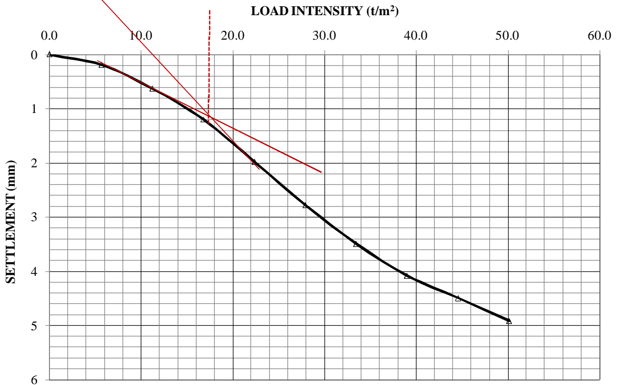
LOAD INTENSTIY v/s SETTLEMENT PLOT
